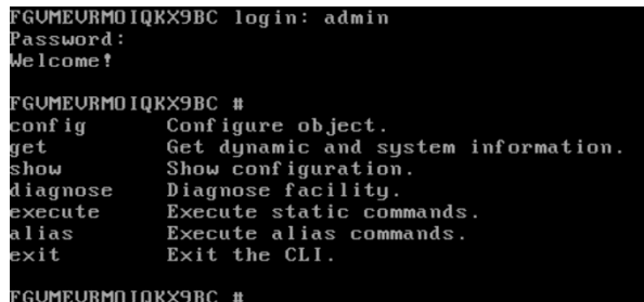
Figure 2: Command Line Help Interface to Firewall Settings and Configuration
