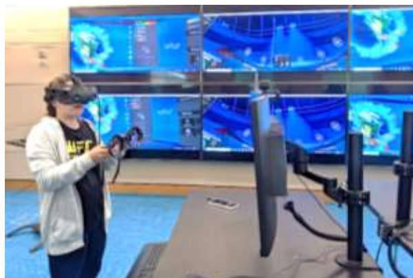
Figure 6. A tethered VR headset is connected to a high-powered workstation.
