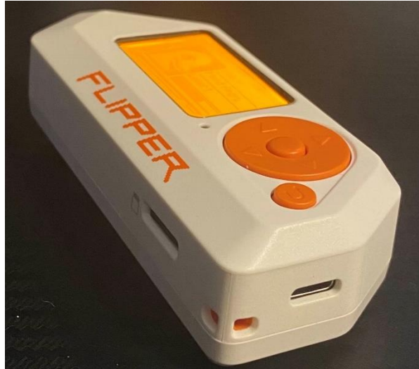
Figure 2: The Flipper Zero™ – note the MicroSD card slot and USB-C port.
