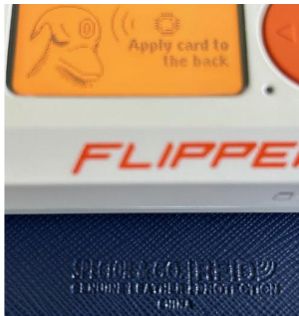
Figure 17: RFID blocking wallet successfully protects smart card.
