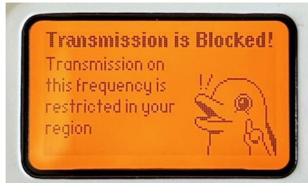
Figure 19: Garage door signal cannot be broadcast
