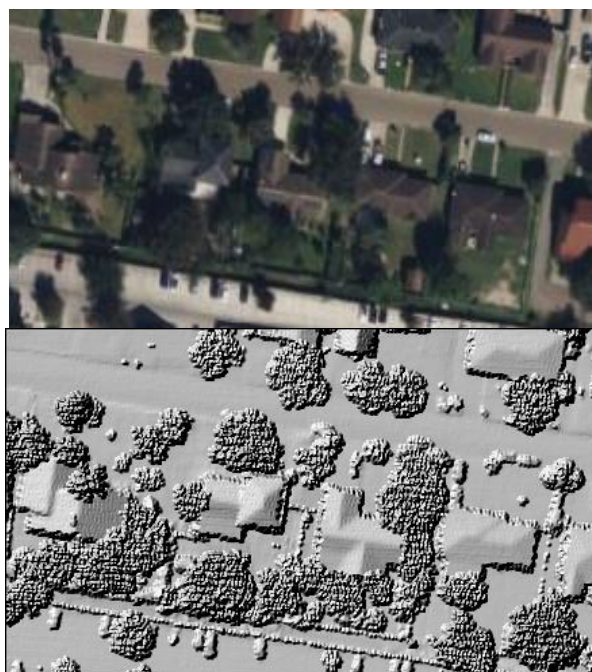
Figure 5. LiDAR surface view of houses and surrounding trees
