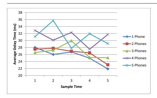
Figure 10: Average delay time of single source audio stream network (100 Packets)
