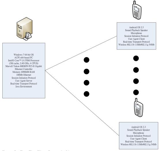
Figure 3: Two-Tier Client Server Architecture
