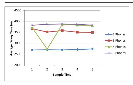
Figure 12: Average delay time of multi-sources audio stream network
