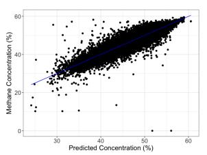
Figure 4. Predicted methane concentration of the LFG vs the actual methane concentration.  $R^2$ =0.9032.
