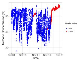
Figure 2. Displays LFG methane concentration at Rockingham County Landfill from 1 Oct 2012 to 31 Nov 2012.
