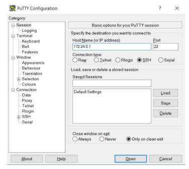
Figure 4. SSH connection to raspberry pi
