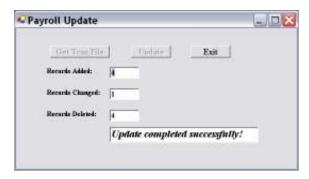
The COBOL proxy program receives the transaction file name and places it into its linkage section. Then the proxy program calls the COBOL legacy program, sending the transaction file name and receiving back the update statistics: records added, changed, deleted, and a completion message. These statistics are then placed into the data object, which is returned back to the C# program.
