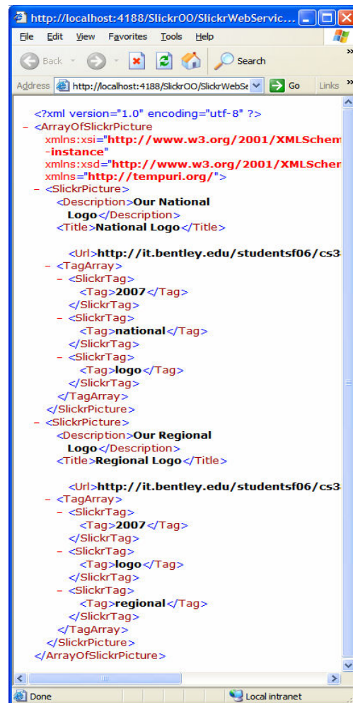
Figure 7. Testing a Web Method and examining the XML-formatted data it returns.
