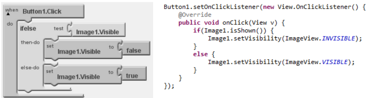
Figure 4: Handling the event of a button clicked using Visual code (left) and Textual code (right) (Soares, 2014, p. 58).
